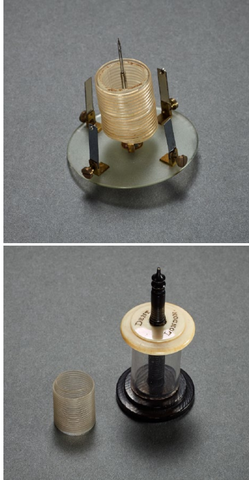
Figure 2(a). (Top) Glass balance-spring attached to glass balance disc, dated: 1836, previously incorporated into a chronometer and trialed, British Museum No. 1976,0202.69. The Trustees of the British Museum (CC BY-NC-SA 4.0).
