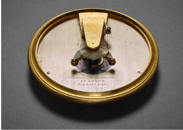
Figure 1. Flat spiral balance-spring made of glass fixed to three-ball mercurial balance. British Museum No. 1958,1006.3073. The Trustees of the British Museum (CC BY-NC-SA 4.0).
