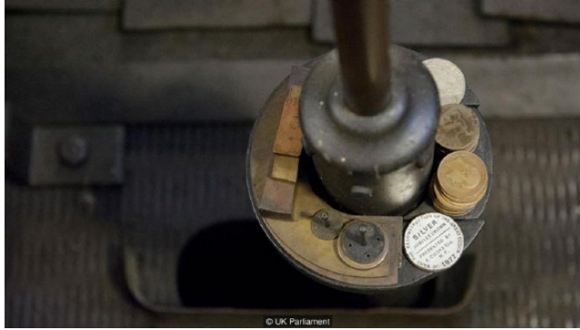
Figure 13. The pennies used to regulate Big Ben's going rate, with one penny producing a gain of approximately two-fifths of a second in 24 hours. Copyright: UK Parliament.
